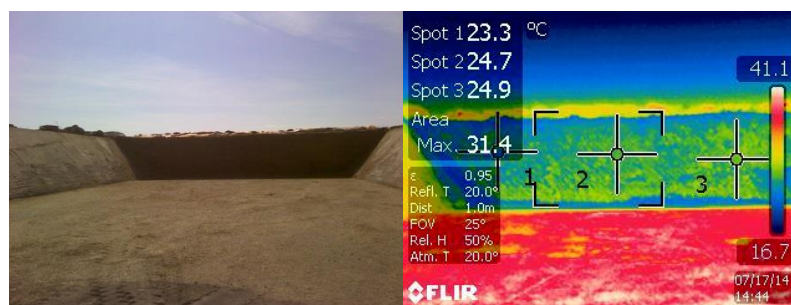
Figure 4: Stable silage. The infrared picture on the right corresponds to the silo front on the left. Temperature from top to bottom (circles 1, 2, 3), are 23.3, 24.7 and 24.9°C respectively (ambient temperature 20° C)
